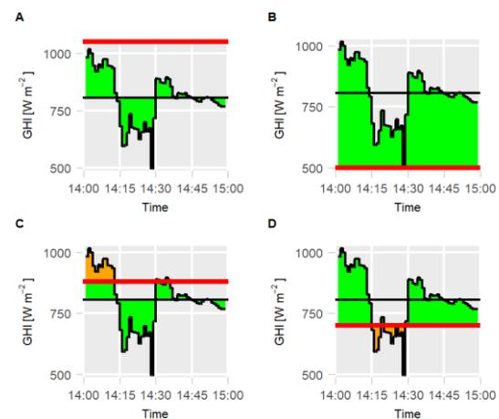
**Figure 1:** Irradiance evolution within one hour. On the left (cases A and C) the clipping threshold is above the hourly average, on the right (B and D) it is below. In the top row (A and B) the hourly averaging will capture correctly the clipping losses, while in the lower row (C and D) the clipping losses will be underestimated by an amount proportional to the orange surfaces.
