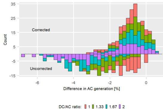
**Figure 8:** Histogram of the distribution of errors comparing the yearly AC generation from the hourly simulations with that of the minute simulations. All cases (site, orientation, and DC/AC ratio) have been considered. The distribution of errors without correction is shown as negative counts, the one with correction as positive counts. Different DC/AC ratios are shown in different colors.
