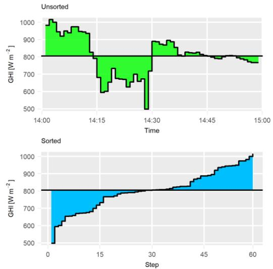
**Figure 3:** Re-ordering the minute values within an hour does not affect the simulation results. Sorting the values in ascending irradiance values allows to describe the irradiance value distribution with a simple approximation.
