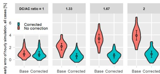
**Figure 9:** Violin plot of the distribution of errors, comparing comparing the yearly AC generation from the hourly simulations with that of the minute simulations. The different DC/AC ratios have been separated and corrected vs. uncorrected results are shown side by side. Central points denote the median of the distribution and the error bars show the 25% and 75% quantiles.
