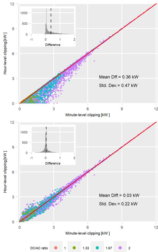
**Figure 7:** Comparison of the clipping losses of the hourly simulation with the hourly sums of the minute simulation for a 9kWAC PV system and four different DC/AC ratios. The first plot uses values without correction, while the second plot uses the corrected values.
