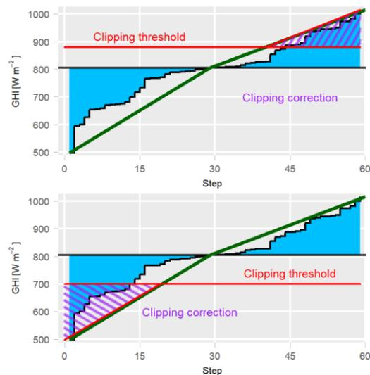
**Figure 4:** Approximation of the ordered irradiance values by two stretches of straight lines. The lines are delimited by minimal and maximal irradiance, and touch at the point where the values cross the mean. The clipping correction is approximated by the area of the textured triangle.
