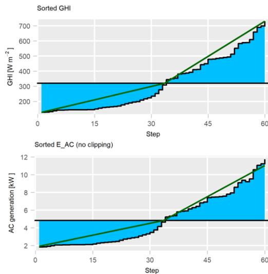
**Figure 5:** When going from global horizontal irradiance to generated AC power, the shape and ordering of the minute-level values changes. The simple linear approach uses just a linear rescaling of the two straight lines.
