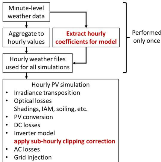
**Figure 2:** Approach for correcting the sub-hourly clipping losses. When aggregating the minute-level weather data to hourly values, additional coefficients are stored together with the hourly values, and which are used in the inverter modeling to estimate the sub-hourly clipping losses.
