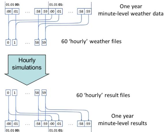
**Figure 6:** Decomposition of one-minute weather data into 60 'hourly' files. Each of the files is used as input for one hourly simulation and the results are re-assembled to give an effective one-minute simulation.
