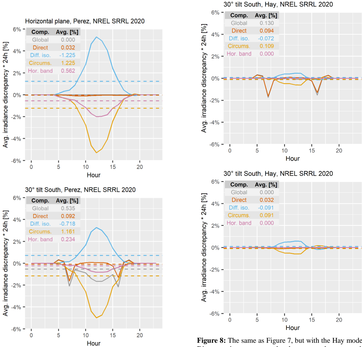
Figure 7: Daily profile of the discrepancies for different irradiance components with the Perez transposition. An average for the whole simulation by hour of the day has been taken. Once transposed, components that compensated each other in the horizontal plane now generate a bias.
