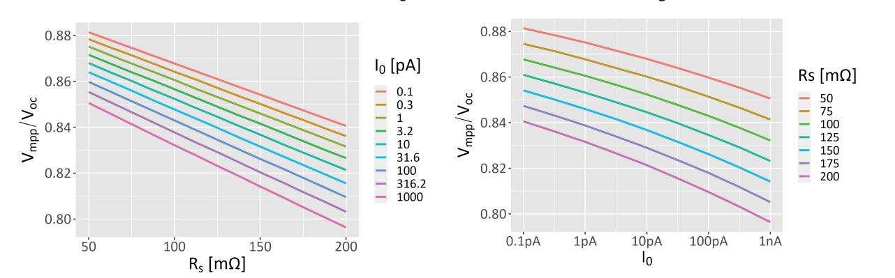
However, changing  $R_s$  and  $I_0$  impacts on other results of the one diode model, like  $V_{mpp}/N_{cells}$  and the low light efficiency. A realistic description of a PV module, should make sure that these quantities stay within typical limits.
