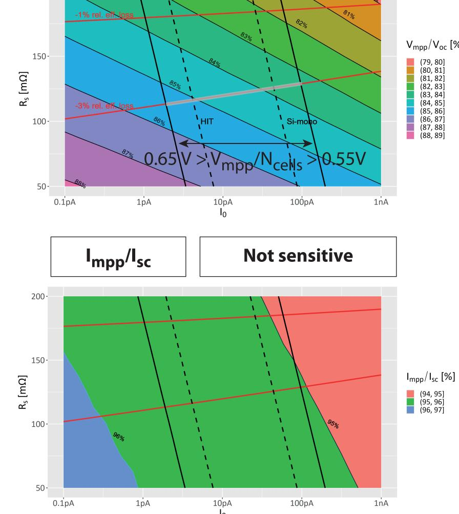
For V<sub>mpp</sub>/N<sub>cells</sub> between 0.55V and 0.65V and a relative efficiency loss of 3% at 200  $v_{mpp}/v_{oc}$  [%] W/m2 the ratio  $V_{mpp}/V_{oc}$  is limited to values between 83% and around 85%. (82, 83] The limit at 85% implies very small satu-
