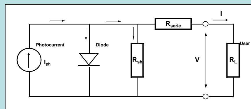
The model has to pass through the 3 special points  $(0, I_{sc})$ ,  $(V_{mp}, I_{mp})$ ,  $(V_{oc}, 0)$
