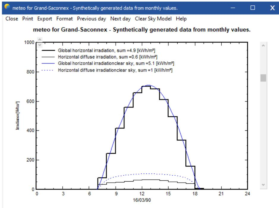
However, this may be different for personal data that is imported with the "custom files" tool. If the data does not match the Clear sky model and are shifted toward morning or evening, this indicates that the time stamps of the data does not match the PVsyst standard and all the models using solar geometry will not work properly.
