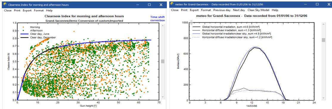
The third control plot “Best clear days Ktcs” displays the sorted Ktcs of all days of the year. The Ktcs is the clearness index referenced to the clear day model (not to the extraterrestrial). This graph gives an idea of the calibration of the irradiance sensor: the best days of the data should be close (within 5%) of the clear sky model, i.e., Ktcs=1.
