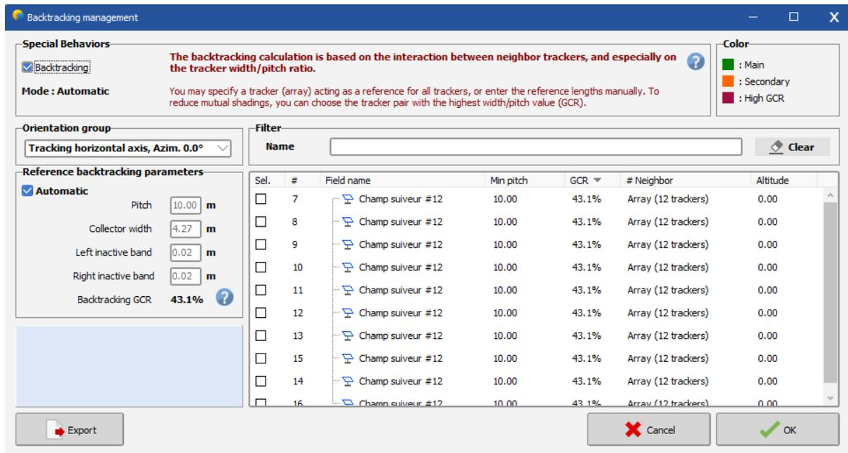
This tool lists distances between neighbouring trackers in descending order. Selecting a tracker with the highest ground coverage ratio (GCR) allows for a recommended neighbour tracker (highlighted in orange) to associate with. Users can set backtracking reference parameters automatically or select specific tracker fields in the list.
