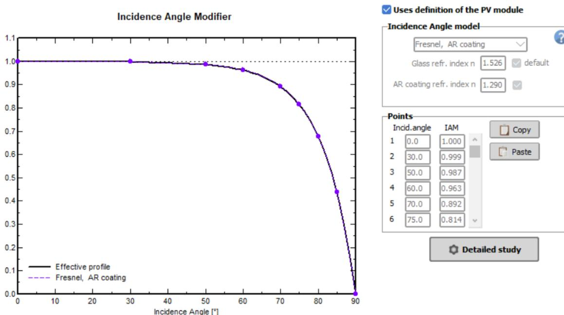
The IAM model is defined with the PV module parameters, page *Additional data, Customized IAM*. If the IAM curve is highly over evaluated with respect to the Fresnel's laws, you will have a warning message while opening the .PAN file. An over evaluated IAM curve could lead to an overestimation of your system's production.
