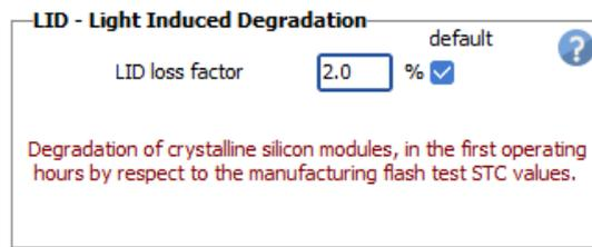
It is very difficult to obtain data about the LID effect on a given module sample. This is never referenced by the manufacturers of course. It depends on the origin of the Silicon wafers, and may vary from product to product, but also may depend on batches of a given production. As it is not sufficiently established, the LID loss is not proposed as default by PVsyst. If you specify it explicitly, the proposed default value is 2%.
