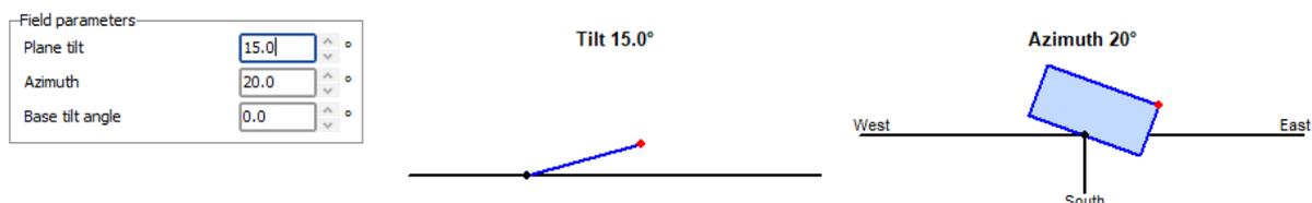
In the fixed planes definition, PVsyst displays a quick optimization tool, indicating the energy yield as a function of the tilt and the azimuth. This is a rough estimation meant for judging how your orientation choice (violet point) will affect the yield with respect to the optimum. This may show the annual, summer or winter yield.
