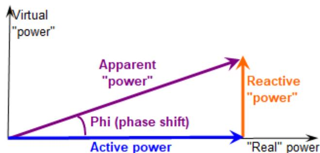
**Lagging reactive power:** When the current lags behind the voltage, with a positive phase angle,  $\varphi > 0$ . Defining a lagging PF in your inverter means the inverter will inject reactive power into the grid to help compensate for reactive power demand of inductive loads such as motors and transformers.
