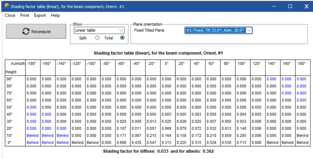
The Shading Factor represents the proportion of the PV field that is shaded relative to its total sensitive area, for a specific sun orientation (where 0 means no shading and 1 means completely shaded).
