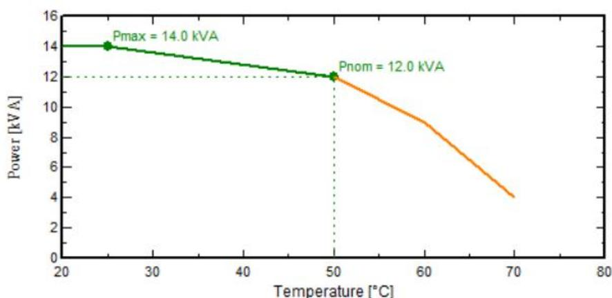
In the simulation, by default the inverter temperature is the external ambient temperature (outdoor installation). This strategy can be modified in Inverter Temperature page in the Energy management.
