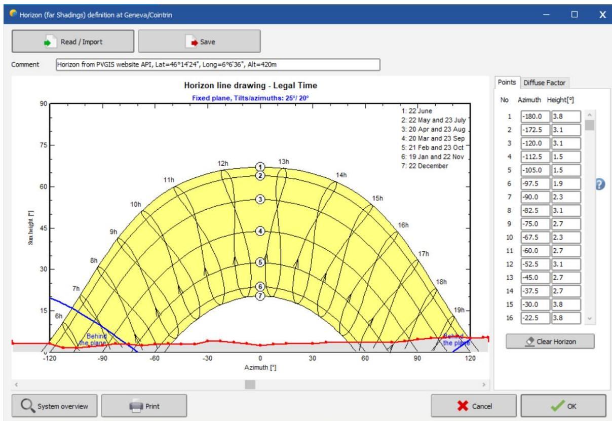
For horizon profiles established using a geo-reference grid (like PVGIS and Meteonorm), the exact location should be carefully defined. You can edit the latitude and longitude in
