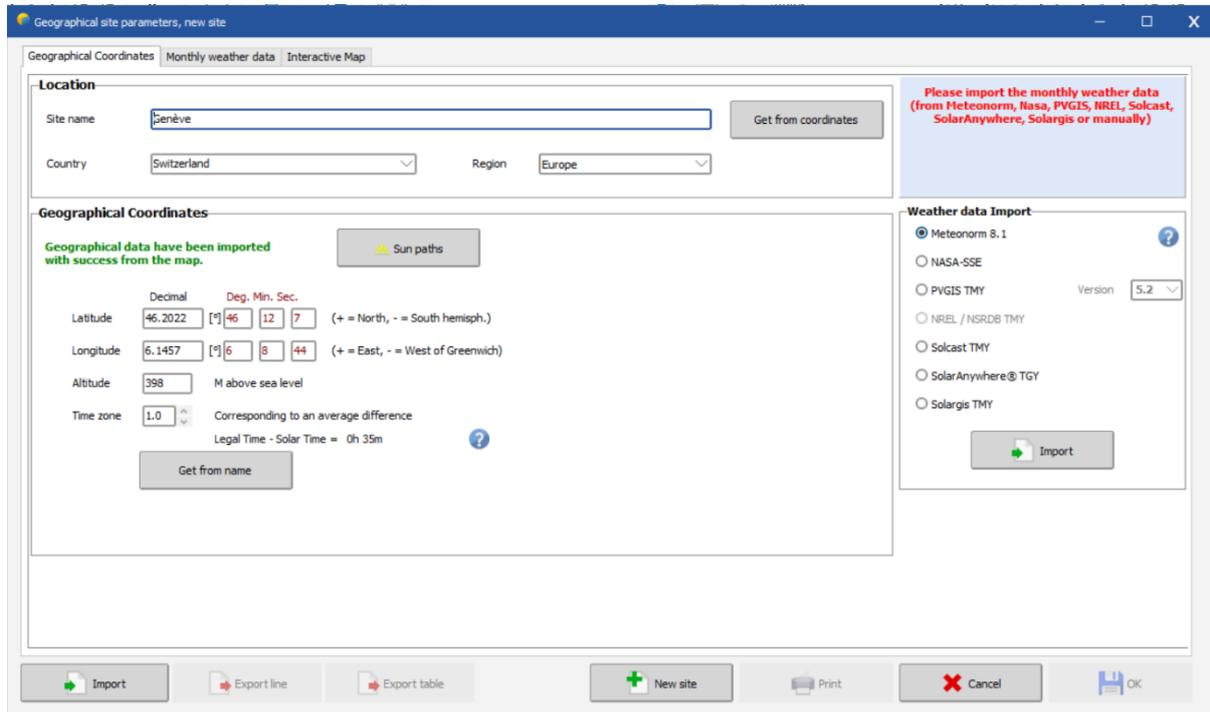
When creating a geographical site, you can directly import **Weather data** from a list of weather data providers, such as Meteonorm, PVGIS, Solcast, Solar Anywhere and Salargis. For the import to work, you need to have a working internet access. The imports are automatic based on the coordinates of your site.
