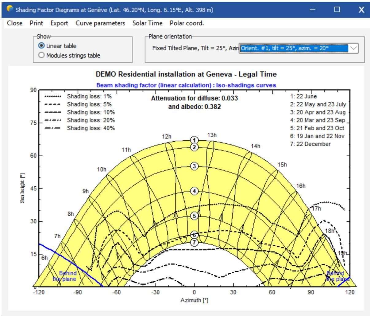
Blue lines on the diagram mark the points where the sun's rays are parallel to the surface. This diagram provides a concise overview of how shading varies with the seasons and times of day throughout the year.
