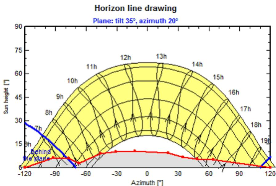
The horizon profile may be defined manually by a set of (Azimuth/Height) points in degrees. These may be from on-site measurements (using land-surveyors instruments like compass and inclinometer). They can be imported from several sources, either as a
