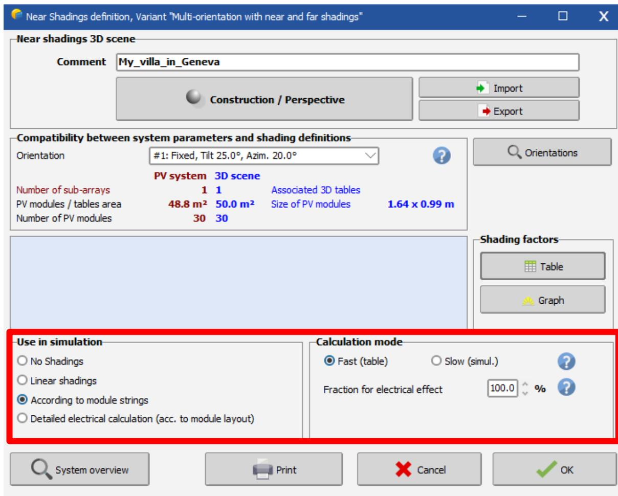
For a more precise result, you can specify the electrical effect fraction from "pure linear" calculation (fraction for electric effect of 0%) to full electrical effect (fraction for electric effect of 100%).
