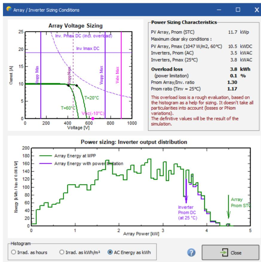
When designing the array, the number of modules in series has to stay within the requirements of
