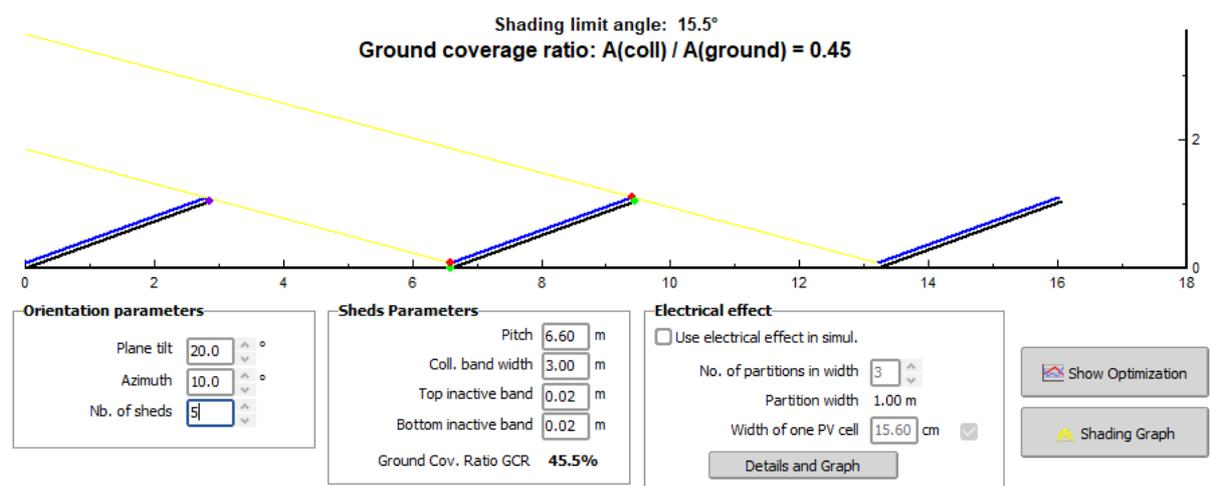
The ground covering ratio (GCR) and the limit angle (the profile angle for which you begin to have mutual shadings) is calculated based on the parameters you choose and shown in the top of the window. As there are shadings, this tool also allows for some advanced options to define number of partitions for the calculation of the electrical shading effects.
