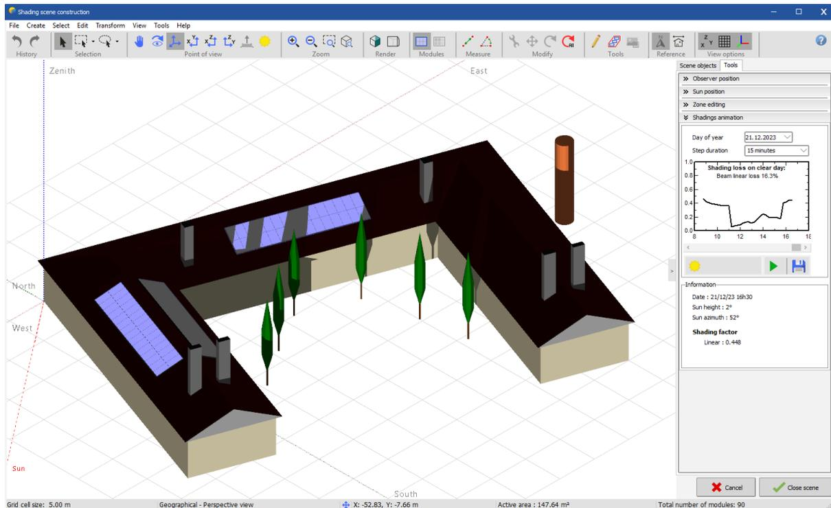
For example, the linear shading on PV module surfaces on December 21 is 16.3%.
