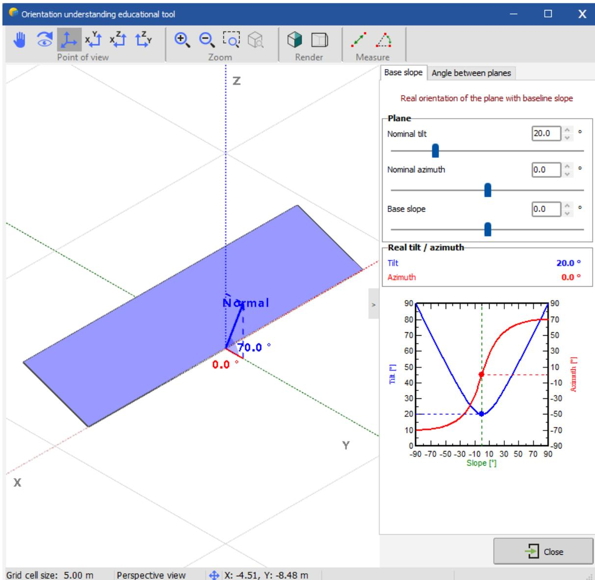
In the **Base slope** tab, users can view a PV table with an initial orientation and apply a base inclination, such as ground slope, to see the resulting tilt and azimuth. Users can experiment by inputting a "Nominal Inclination," "Nominal Azimuth," and adjusting the "Base Inclination," potentially representing terrain slope, to observe the final tilt and azimuth after applying the base inclination.
