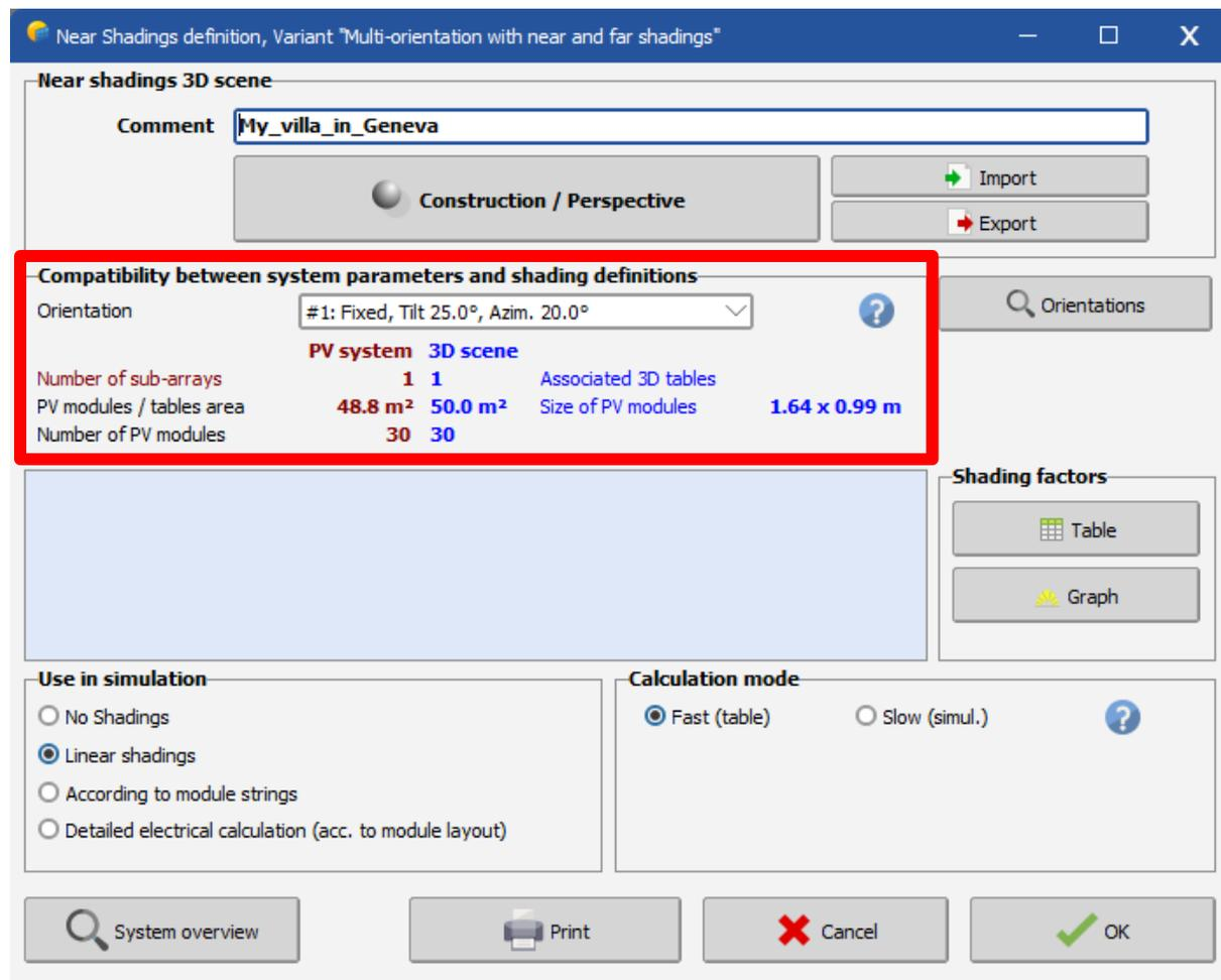
First, there is a dropdown list for the different existing orientations. Next, information about the number of sub-fields, the surface area of existing PV modules, and, finally, the total number of PV modules is displayed.
