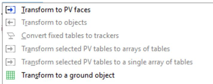
**Transform to PV Faces:** Selected faces can be transformed into a PV surface.
