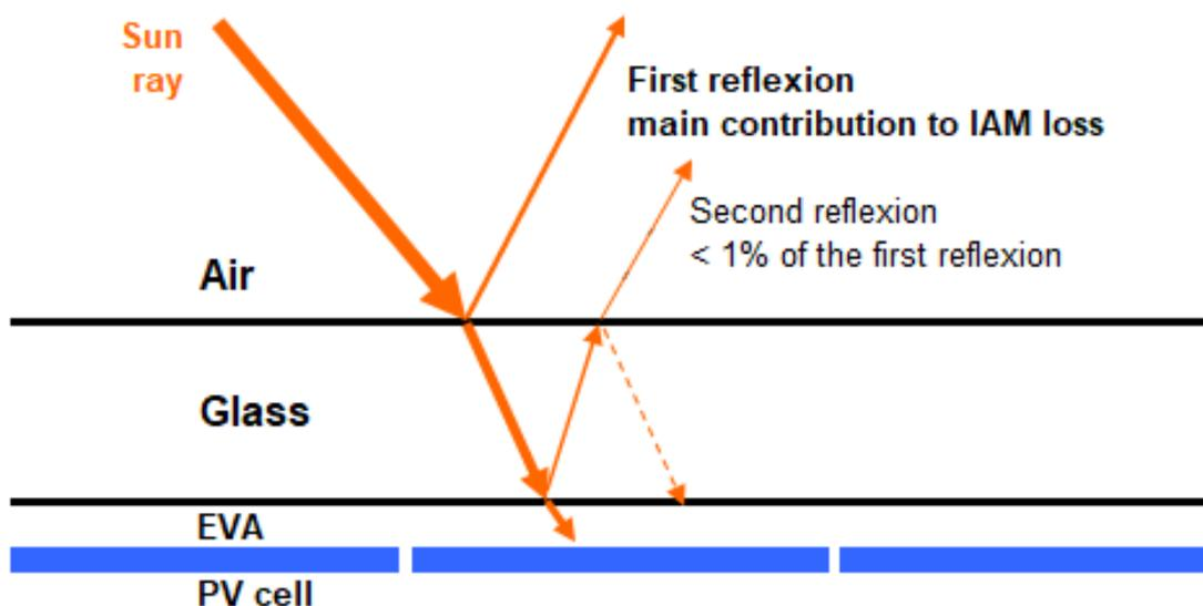
PVsys uses an IAM function, which describes the deficit of transmission as a function of the incidence angle. This function is applied to the beam component, and to the diffuse and albedo, using an integral over all *seen* directions, supposing an isotropic distribution of the diffuse irradiance.
