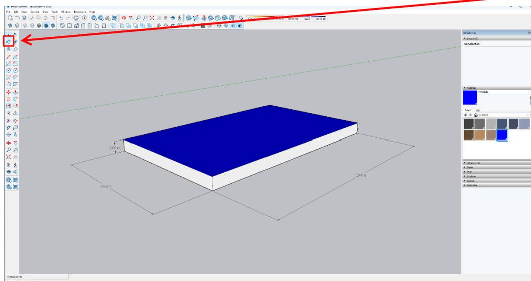
Figure 5 : Colouring the surface of the PV module in SketchUp
