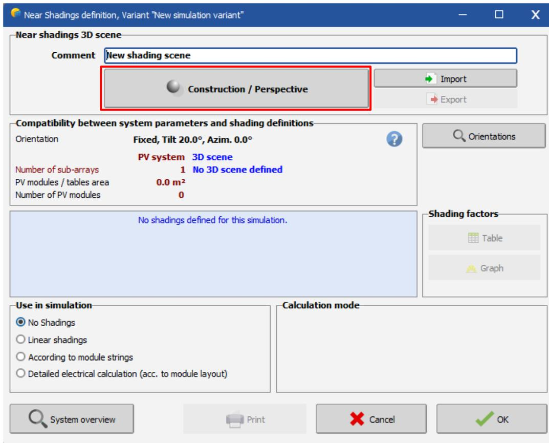
Figure 41 : "Near shading" window
