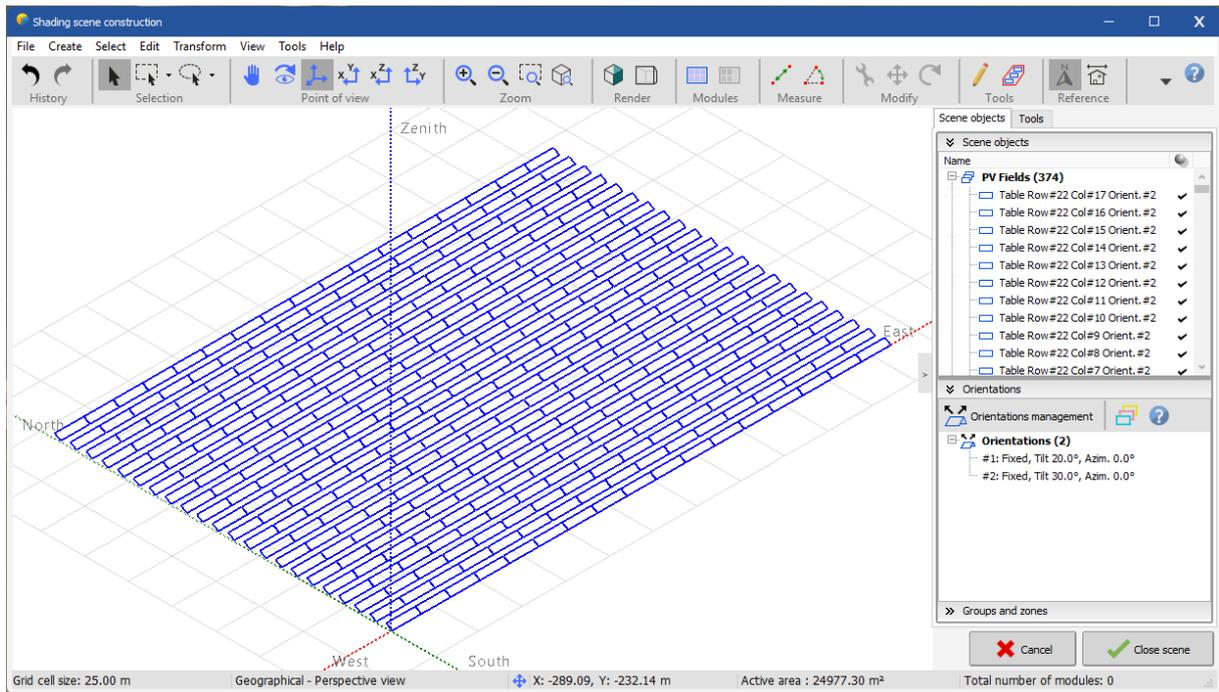
Figure 56 : PVC imported into the shading scene
