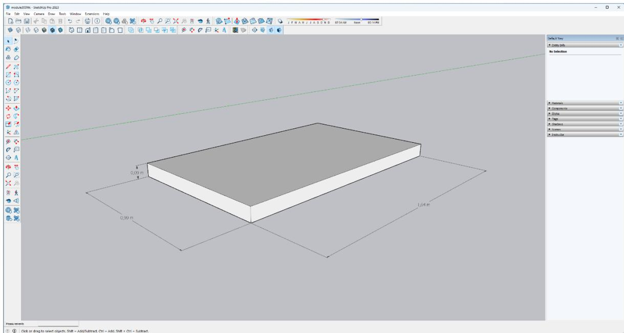
Figure 2 : 3D scene of a PV module in SketchUp
