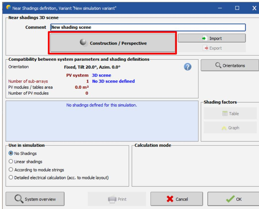
Figure 52 : PVsyst dialog to define shading
