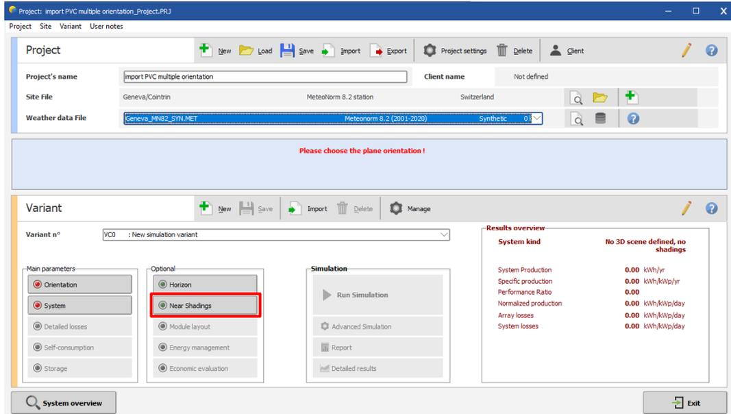
Figure 64: Pvsyst window for multiple orientation import
