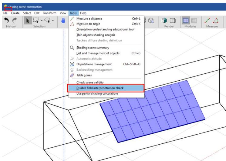
Figure 19 : Deactivate the verification of field interpenetration in PVsyst
