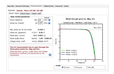
This page summarizes other parameters, as calculated when establishing the one-diode model.
